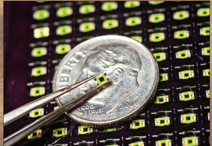
Semprius modules use hundreds of GaAs solar cells with lenses to concentrate light, boosting the efficiency and making the exotic photovoltaic affordable
