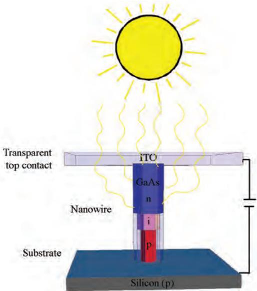
Above, the sun's rays are drawn into a nanowire, which stands on a silicon substrate. At a given wavelength the sunlight is concentrated by up to 15 times (Credit: Niels Bohr Institute)
