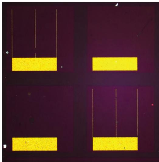
Optical microscope image of NW solar cells
