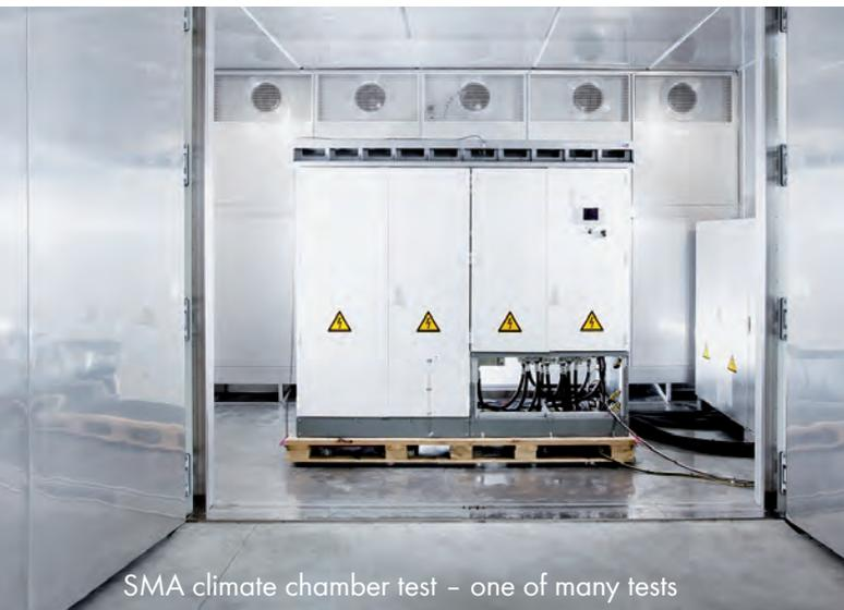
SMA climate chamber test – one of many tests
