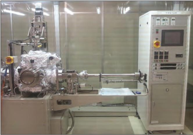
The surface-activated bonding tool involves the bombardment of substrates by a beam of fast argon atoms
