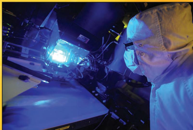
An operator inspects a photolithography tool used to manufacture high-efficiency Solar Junction concentrator solar cells. NREL's pioneering multi-junction work led to the Solar Junction SJ3 solar cell with tuneable bandgaps, lattice-matched architecture, and ultra-concentrated tunnel junctions. (Credit: Daniel Derkacs/Solar Junction)
