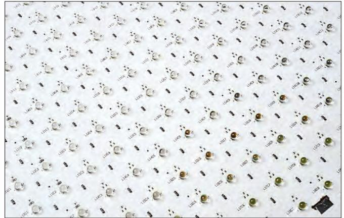
The GaAs is the black square on each cell; Semprius's micro-transfer printing process is poised to make these exotic solar modules cost effective
