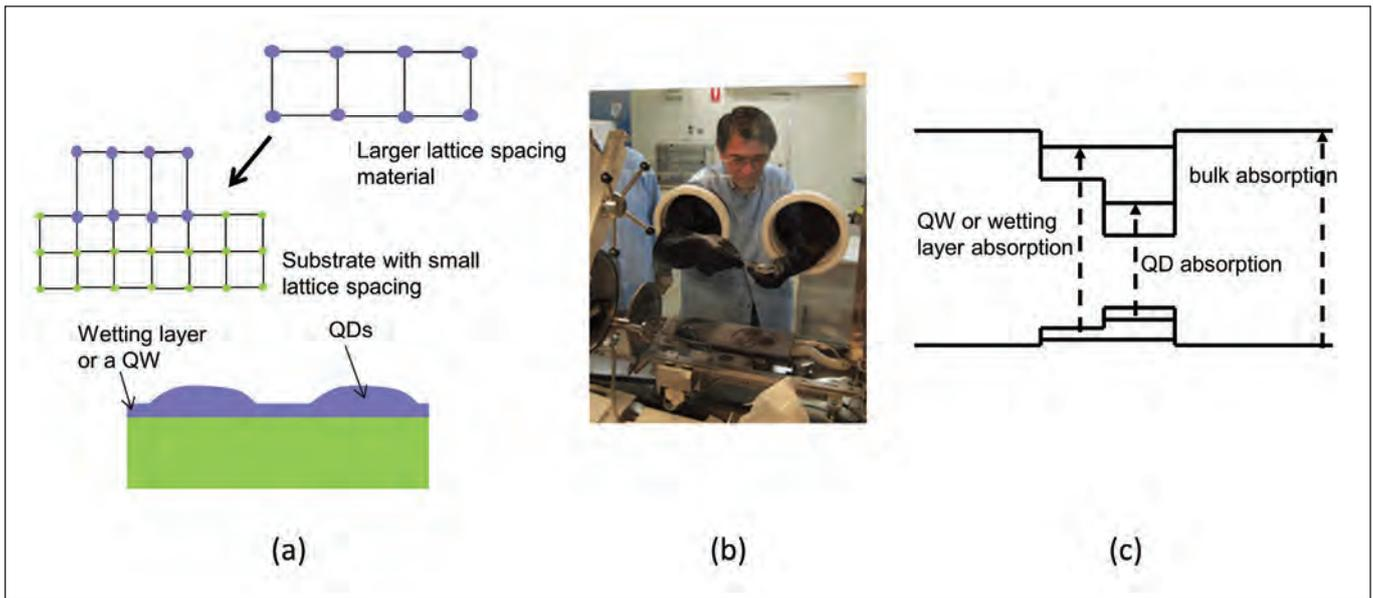
Figure 1: The formation of quantum dots in the Stranski-Krastanov growth mode (a) and the MOCVD reactor used for growing QWs/QDs (b). The relative bandgap energies of  $\text{In}_x\text{Ga}_{1-x}\text{As}$  quantum dot and quantum well (or wetting layer) with respect to bulk GaAs (c)
