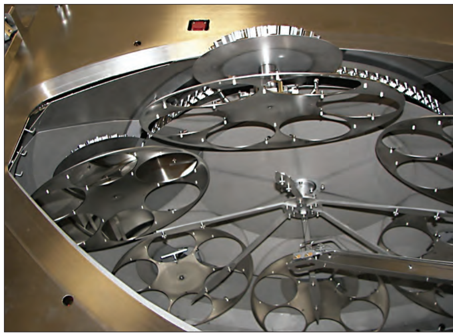
Figure 7. Higher levels of film thickness uniformity are possible by switching from a single-axis tool to one that provides dual axes of rotation. An example of the latter is the Temescal UEFC-5700, which accommodates 36 wafers in six domes, each holding six wafers
