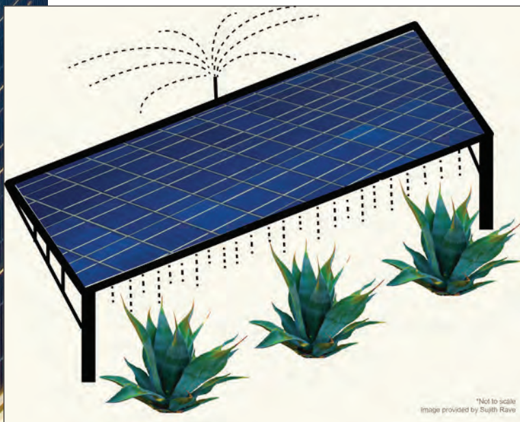
On a co-located solar farm, runoff from water used to clean photovoltaic panels would nourish agave or other biofuel crops. The plants would in turn provide ground cover, helping prevent dust buildup that decreases solar panel efficiency. (Courtesy Sujith Ravi)
