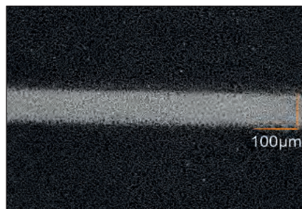
Fig. 3: Ablation of passivation layer with picosecond laser (microscope image) Laser implementation in an innovative manufacturing system
