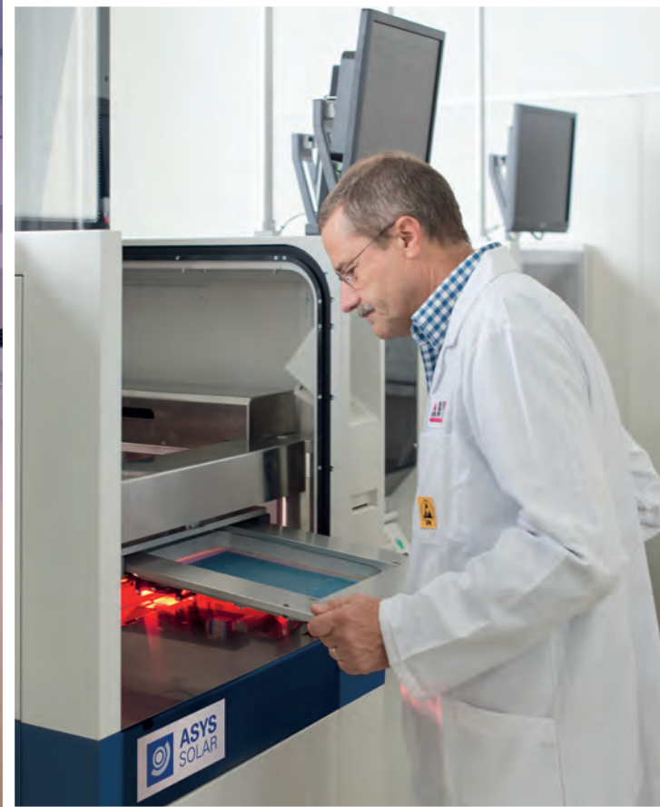
Setting up the XS2 printer. Its new motorized pneumatic print head increases screen life.
