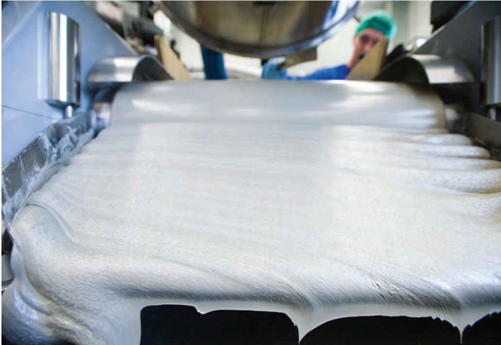
A technician oversees production of new silver pastes at the Heraeus West Conshohocken, Pennsylvania (USA) facility.
