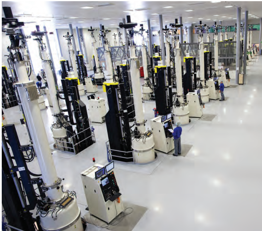
Figure 3. CZ furnace hall Photograph courtesy of Norsun, Norway
