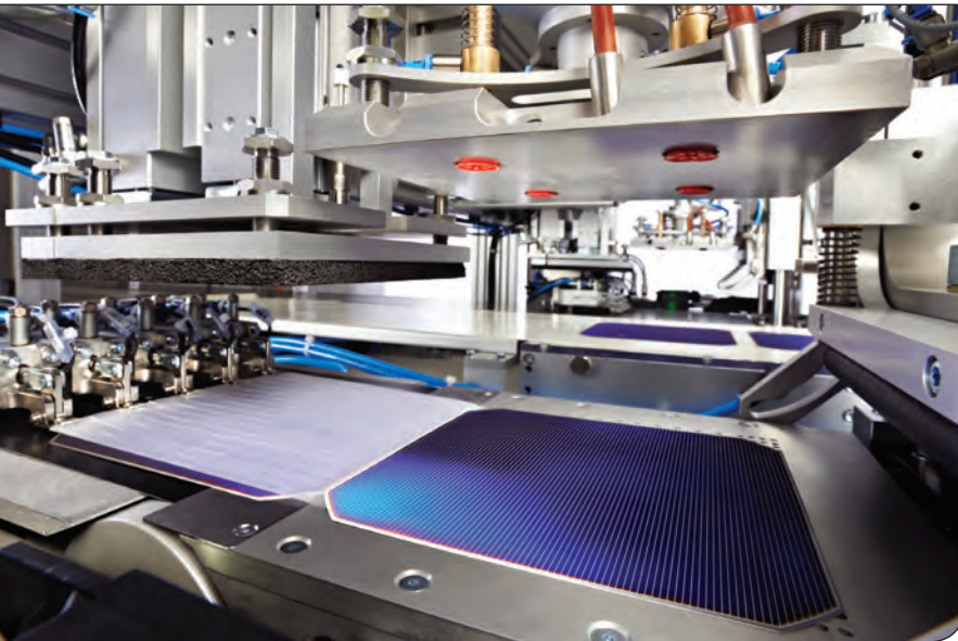
Cell connection station for SmartWire Connection Technology. Image courtesy Meyer Burger
