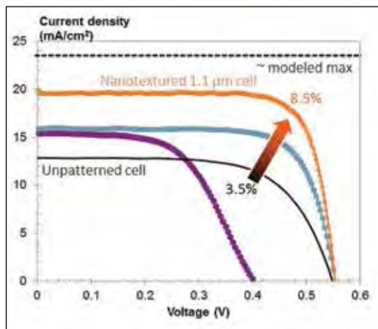
Successful integration of a nanophotonic structure into a 1.1 micrometer c-Si cell. The efficiencies are the highest achieved for this c-Si thickness. This ultra-thin cell is however too thin to be competitive.
