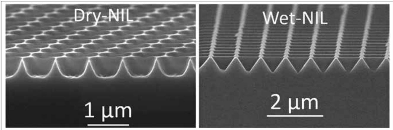
(Left) Dry etching vs. (right) wet etching of the nanopatterns.
