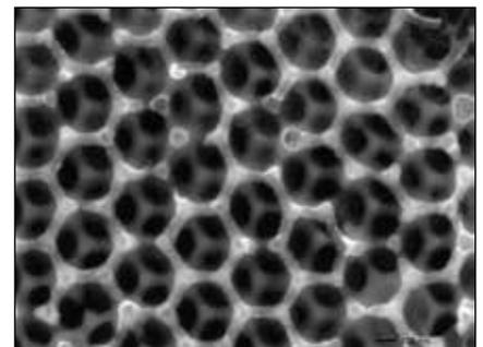
Electronmicroscopical image of the germanium-structure after removal of the polymer templates
