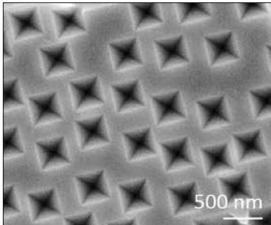
Experimentally introduced disorder via hole-mask colloidal lithography
