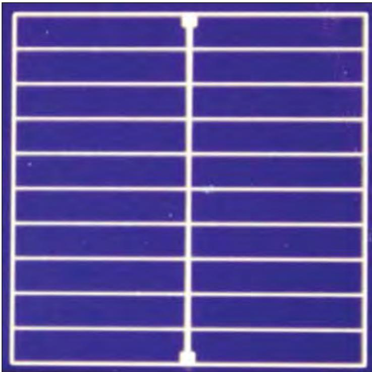
A photo of the DASH (dopant free asymmetric heterocontact) solar cell developed through an international collaboration. (Photo credit: James Bullock/Berkeley Lab, UC Berkeley, ANU)
