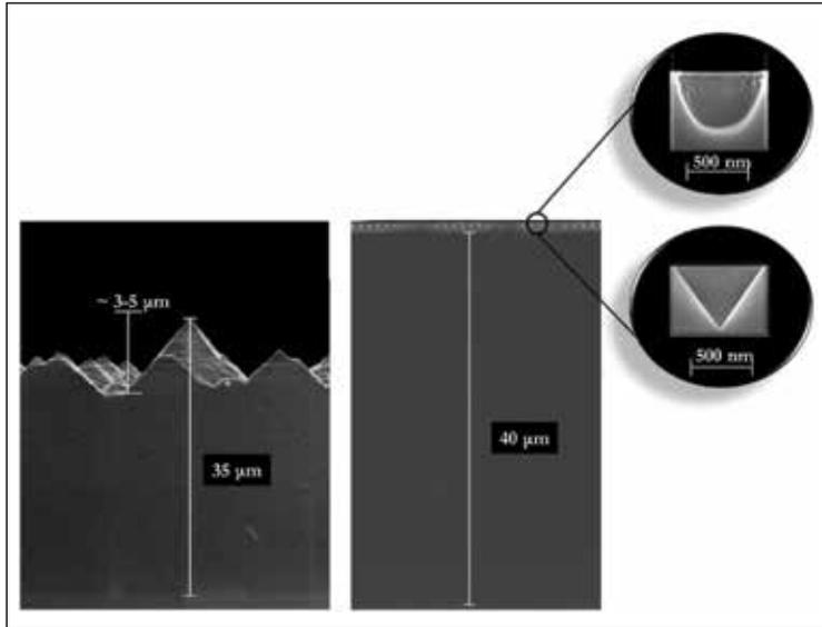
(Left) Micron-scale front-texturing vs. (right) nano-scale texturing, with dry-etched parabolic holes (top inset) or wet-etched inverted pyramids (bottom inset).
