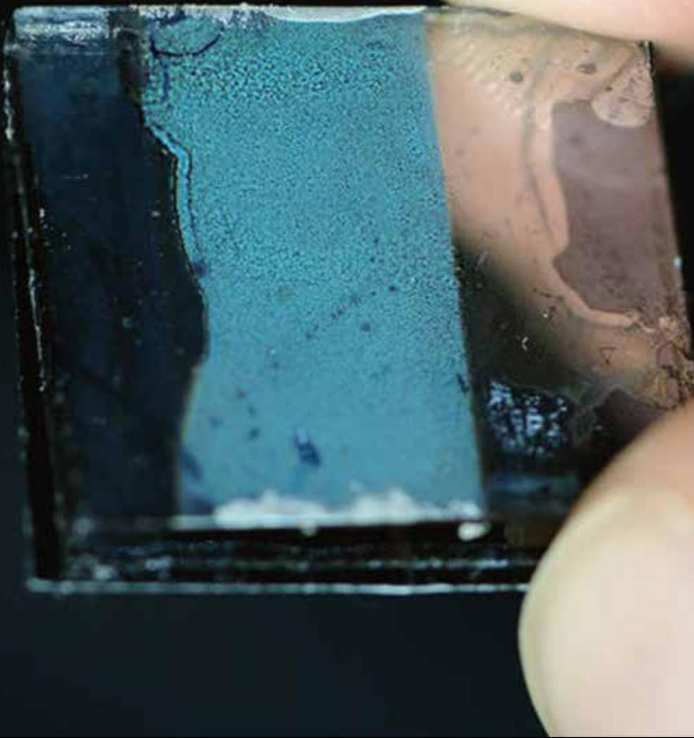
polymer beads form three-dimensional templates in an initial step.
