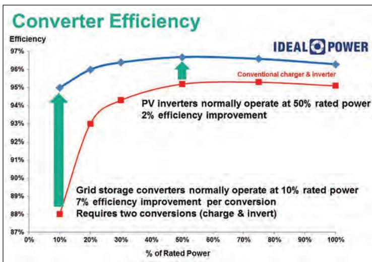
greater for conventional solutions with similar power nameplate ratings. Lastly, PPSA-based systems deliver 10 percent or more in annual OPEX savings due to reduced energy use and simplified Operations and Maintenance (O&M) procedures. Systems using PPSA technology also operate quietly and unobtrusively, a huge benefit for many applications sited behind the meter.
