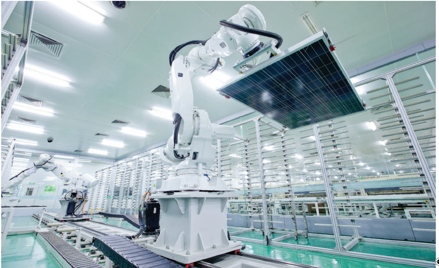
Automation plays an important role across all JinkoSolar plants. Here we see industrial robots handling power binning tasks.
