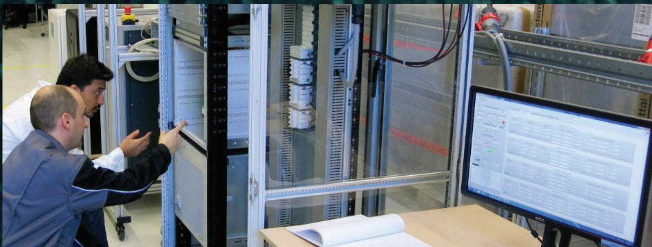
FRAUNHOFER ISE's test rig for home storage systems for self-produced PV electricity. Before beginning the battery tests, the set-up as well as all necessary process steps are checked once again. ©Fraunhofer ISE
